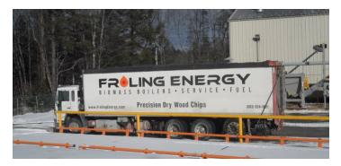
PDCs are blown into the silos from our blower truck
